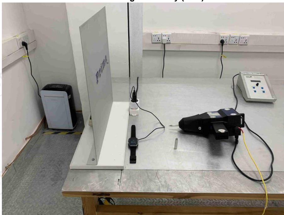
Electrostatic discharge immunity (ESD) test view
