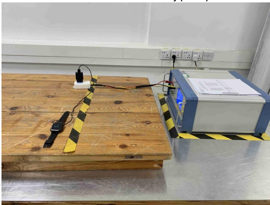
Electrical fast transient/burst immunity (EFT/B) test view
