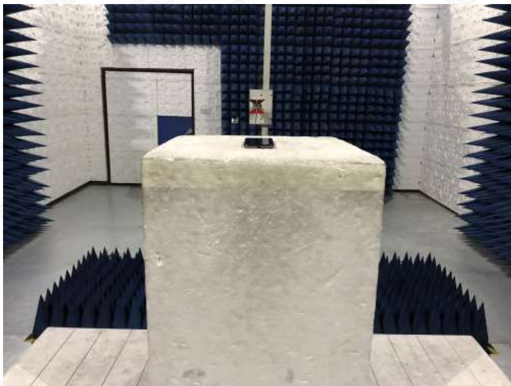
RADIATED SPURIOUS EMISSION ABOVE 1G TEST SETUP
