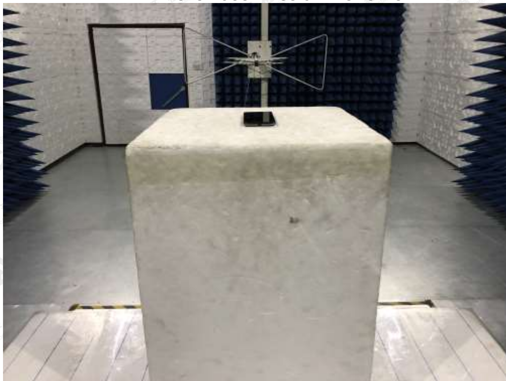
RADIATED SPURIOUS EMISSION-ABOVE 1G TEST SETUP
