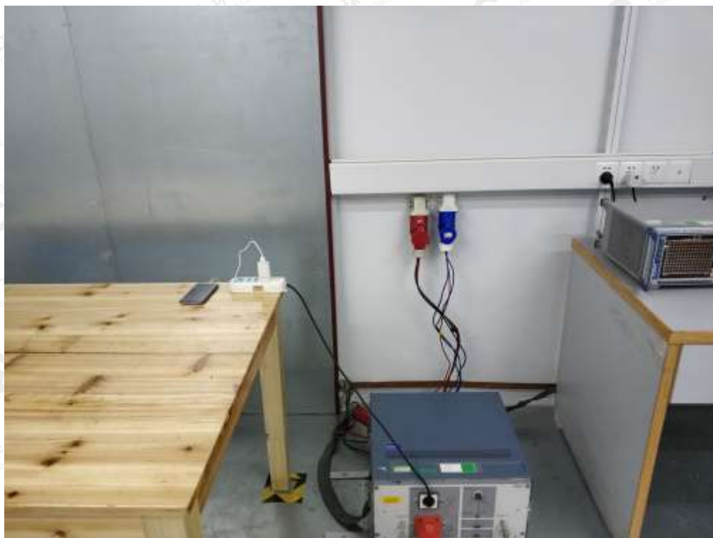
EN 55032 RADIATED EMISSION TEST SETUP
