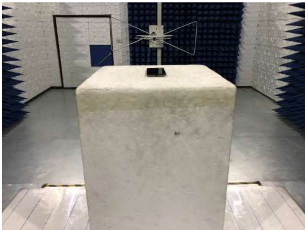
RADIATED SPURIOUS EMISSION-ABOVE 1G TEST SETUP
