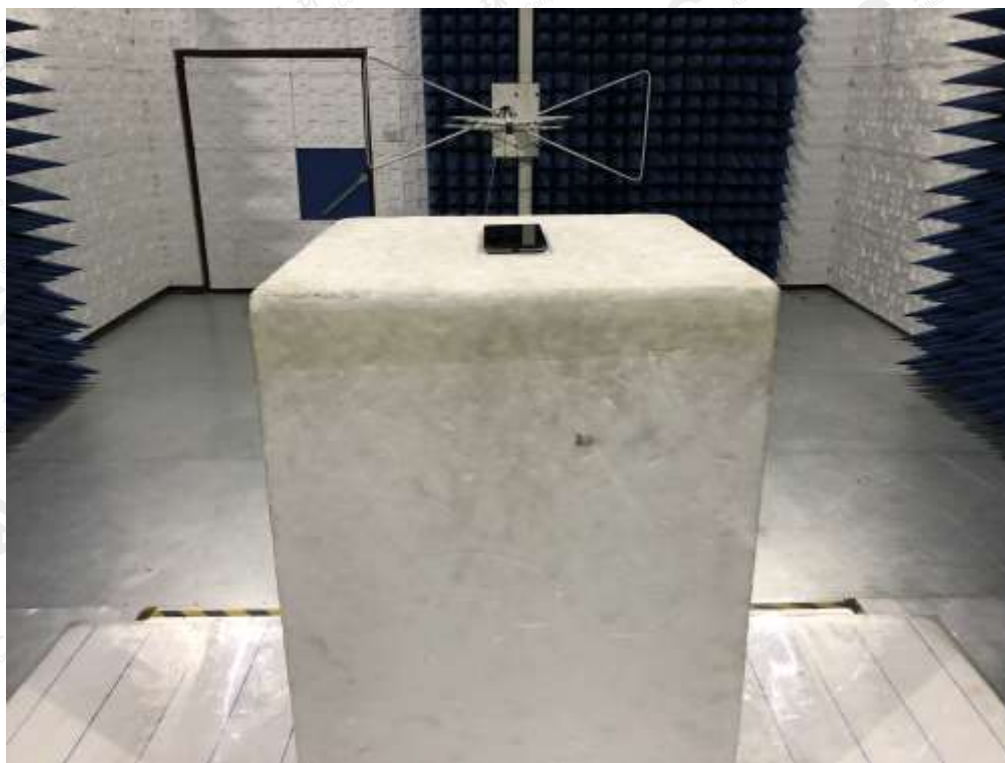
RADIATED SPURIOUS EMISSION-ABOVE 1G TEST SETUP
