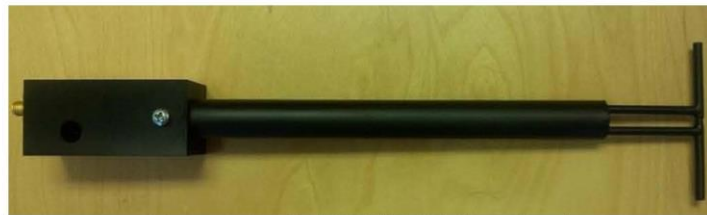
Figure 1 – MVG COMOSAR Validation Dipole
