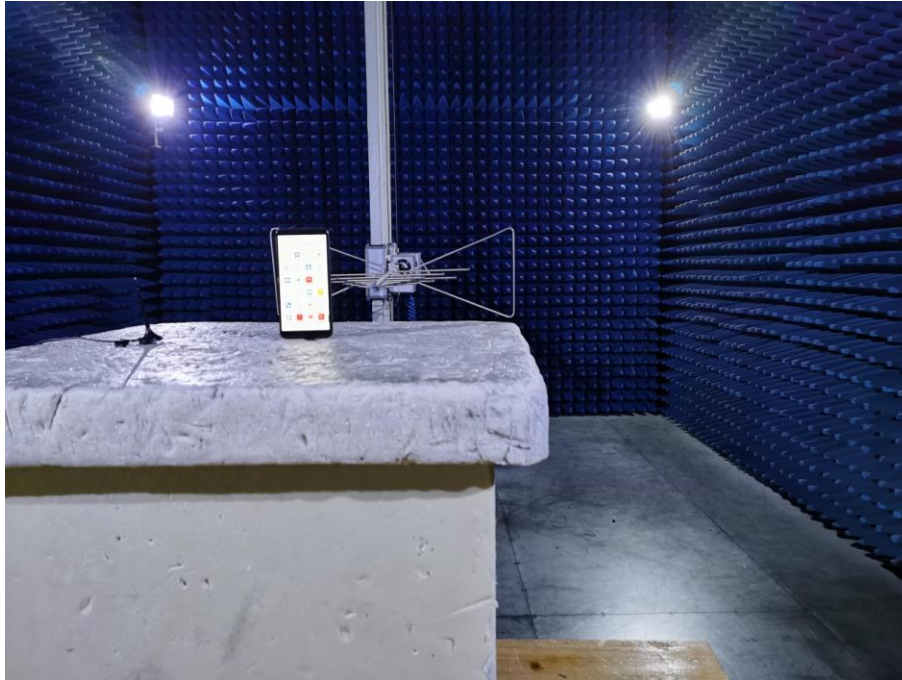
Radiated Spurious Emissions Test View (Above 1GHz)
