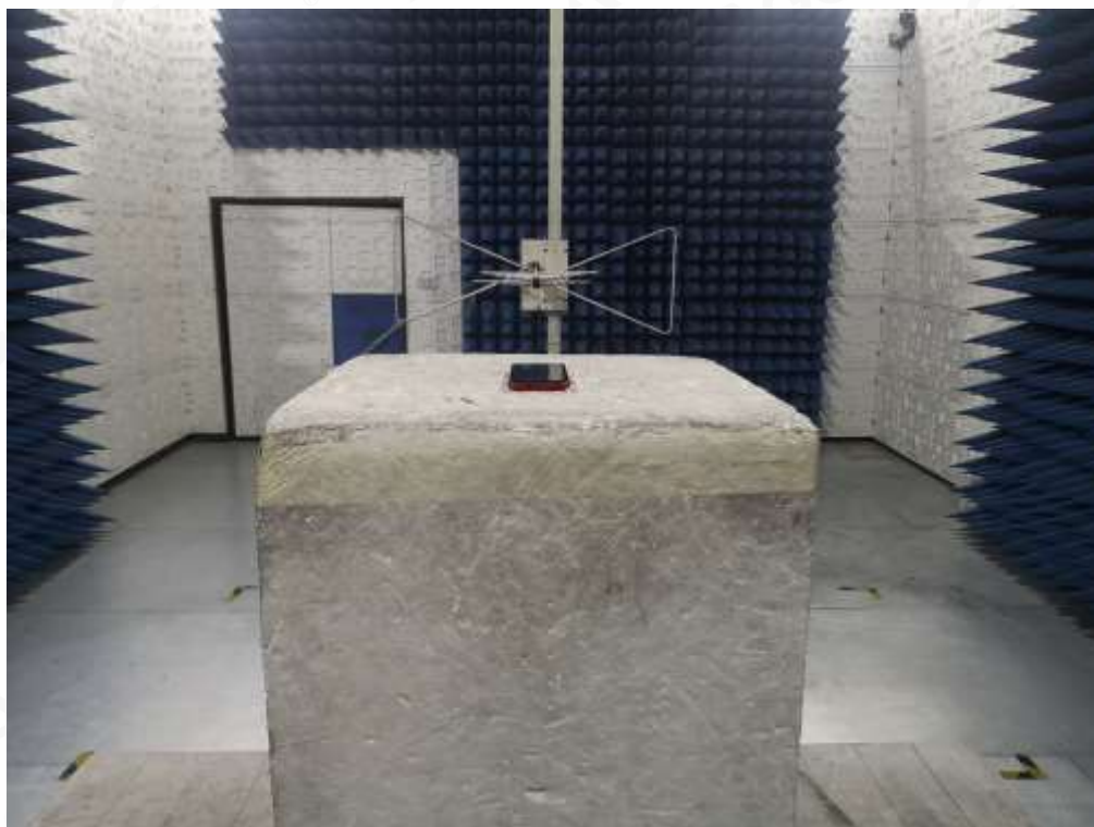
RADIATED SPURIOUS EMISSION ABOVE 1GTEST SETUP
