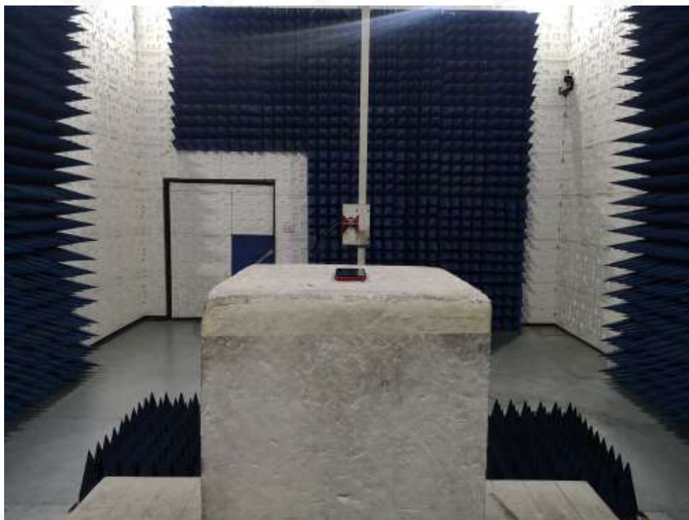
RADIATED SPURIOUS EMISSION ABOVE 1G TEST SETUP
