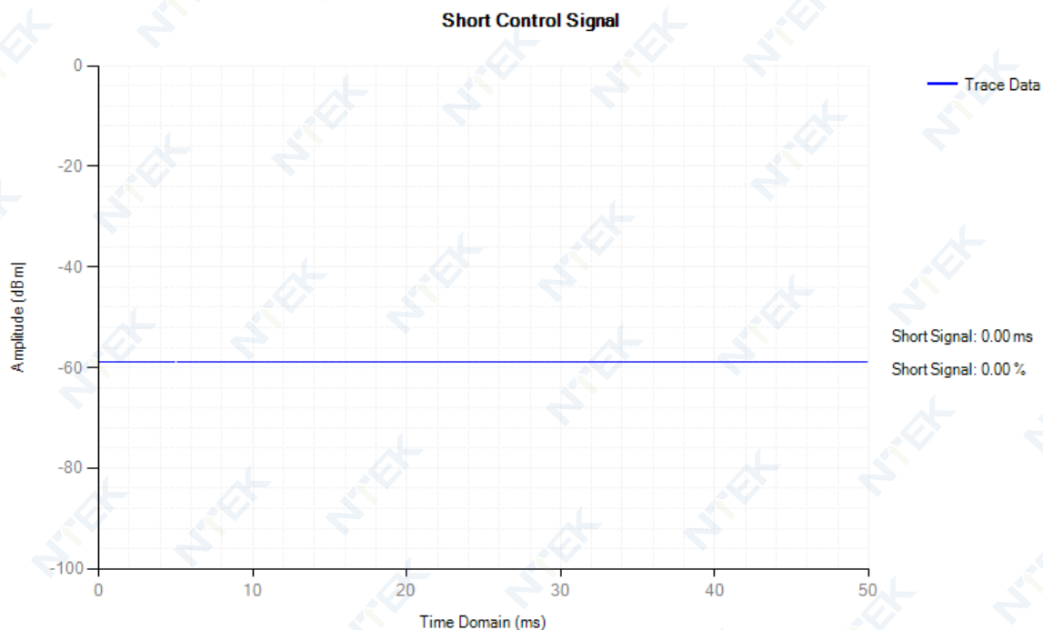
Control Signal NVNT 802.11a 5180MHz AWGN
