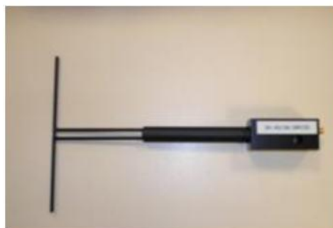
Figure 1 – Satimo COMOSAR Validation Dipole
