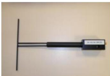
Figure 1 – Satimo COMOSAR Validation Dipole
