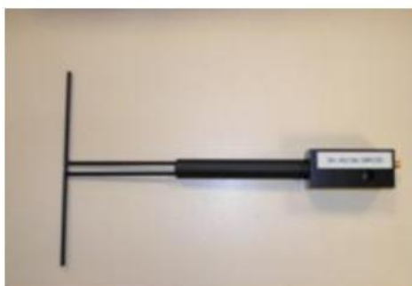
Figure 1 – Satimo COMOSAR Validation Dipole
